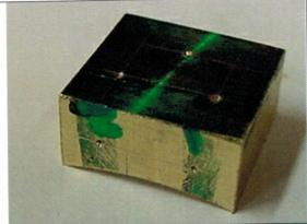
Mark out the various holes in the block. I used a felt marker to provide an easy to see surface for marking. Centre punch and drill holes to depths shown. A depth-stop on the drilling machine helps here. Be careful when drilling through with brass as it has a habit of snatching – use a drill vice, do not try to hold with your fingers, they will lose the argument!
