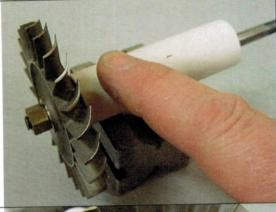
Slide the shaft assembly into the tube and rest it on a raised flat surface - a vee block or even over the edge of your table is fine. Place a finger on top of the tube and rock it back and forth. The turbine will rotate so that the heavy point is downwards.
