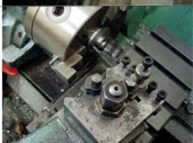
Grip the outside of the Prop-driver and machine the taper in the rear. This angle and shape is not critical as it is to tidy it up and lose some weight. I machined the back taper with a parting tool, considerably extended to get the reach, and took small cuts. You can use your flair to get a shape you like, but don't make it too thin at the centre as it may not grip so well on the taper.
