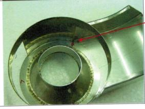
Offer up the right-hand exhaust assembly to the Exhaust Front and Outer, and align the top right hand edge with the epening in the Exhaust Outer – see left.
