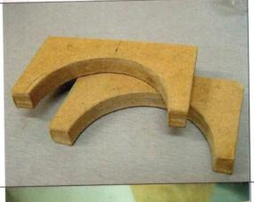
The former is made as two parts from 10mm plywood or MDF about 60mm  $\times$  50mm. A curve of 37.75mm radius is cut into one of the long sides on each piece.
