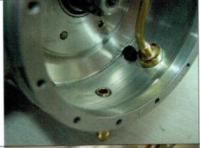
Slide the fibre washer 151, onto the oil drain adapter 167, and smear some liquid gasket compound onto the thread and screw it into the gearbox, securing the manifolds into place.
