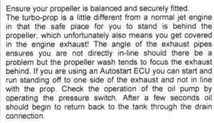
Weight the test stand to ensure it cannot pull over. Ensure you have your fire extinguisher handy for all running and all your batteries are charged (don't forget oil pump cell). Set your ECU to 100,000rpm maximum engine rpm.
