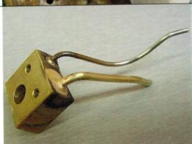
The lube sub-assembly can now be carefully removed and cleaned up to remove flux and get a clean finish. Fine emery paper does a good job in conjunction with a rotary stainless steel wire brush inserted into your "Dremel" to get into the awkward bits.
