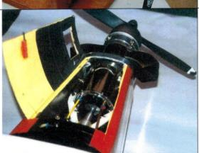
The first prototype turbo-prop to fly was fitted to a 2.4m span "Pilatus Turbo-Porter". This used the power unit secured to a pair of 13mm square aluminium rails, which were subsequently bolted to the airframe. All up weight was 8.2Kg (18Lbs).
