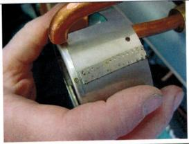
Fit the Exhaust Front onto the Exhaust outer, aligning each component as best you can.
