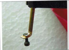
Silver solder an M2.5 nut to the flattened portion of the brass pipe, and seal the flattened pipe end at the same time.
