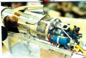
Our second flying plane was a 2m span "Tucano". For this we extended the exhausts slightly to clear the nose and made an extra-long prop-shaft to enable the engine to be sited further into the fuselage. Weight here was 10Kg (22lbs)
