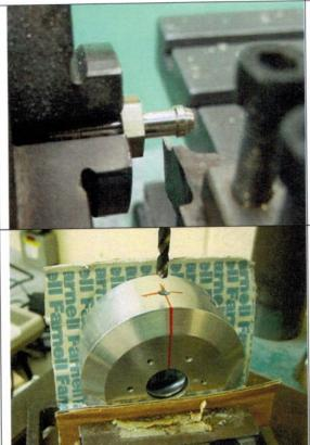
Using a narrow tool, turn the barb which retains the drain pipe. File or turn the chamfer on the end to assist the pipe on when pushing into place.
