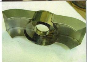
Your exhaust system should now look similar to this. Fit the Spider casting into the Exhaust Outer, this will ensure it is held perfectly circular.
