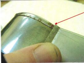
When in position, turn over and check for any overlap over the flanged portion of the Exhaust Front, grind this away if required.
