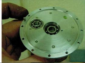
Apply a smear of gasket compound to the rear face of the prop-shaft housing 158, and insert a standard ISO607 bearing to the gearbox front cover to centralise it. Fit the eight M3 x 8mm securing screws 192, apply locking fluid to the threads and tighten firmly.
