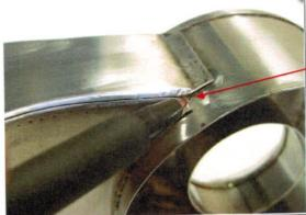
All the seams can now be spot-welded firmly using close spaced welds to achieve reasonable gas tightness.
