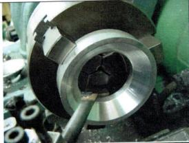
Machine a ring for spinning the outer flange on the exhaust cone, from a bit of scrap aluminium of diameter at least 65mm (ideally 90mm), with an inner hole of 35mm and a slope of 45', tapering out.
