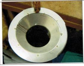
Place the Exhaust Front over the Exhaust Cone and centre. Place a single spot weld and check alignment of the assembly.
