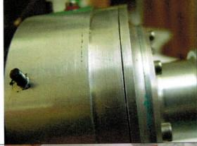
Fit two wavy washers onto the end of the intermediate shaft and ease the front cover into place, ensuring the dowel pin aligns correctly. When there is sufficient pre-load you should find a small gap of approximately 0.5-0.8mm between the front cover and gearbox case. Use a feeler gauge to check the gap.
