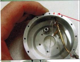
Use a steel rule to point to the M2.5 soldered nut, and sight along this to highlight the location for the drilled hole for the fixing screw, for securing the flattened end of the fitting.
