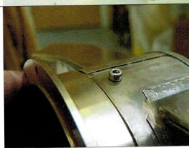
The two exhaust securing holes need drilling in the spider casting. You need to orientate the exhaust so the two exhaust stacks are at 90° to the drain hole in the base of the gearbox. The hole positions are marked on the plan and they should be pre-prepared for you on the laser cut Exhaust Outer, 130.
