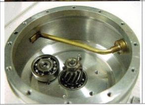
Trim the end of the brass tube to length and flatten the end by reference to the drawing. Clean up the fitting with emery paper to remove scale etc.
