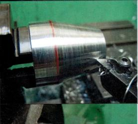
We now need to mount the spinner blank on a mandrel to machine the outside profile.
