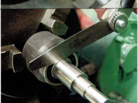
Using a feeler gauge, check the gap in front of the front bearing when the Prop-shaft is pushed fully home on the taper.
