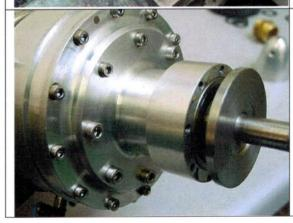
When the prop is first tightened and the power unit is run, the prop driver will lock into place onto the shaft taper.
