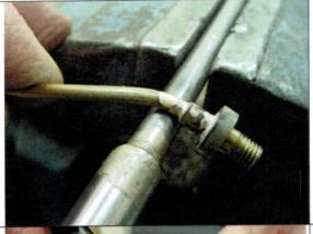
Once soldered, (quench from hot to crack off the flux) the end of the brass tube needs bending close to the fitting.
