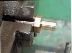
Reverse in the chuck and machine to length of 23mm, and turn the last 9mm to 5.5mm diameter.
