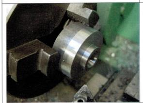
Once the taper is completed, turn the rear boss to 17mm diameter and a length of 4mm. Only do this after the taper is completed as there is plenty of material for you to keep making adjustments if required.
