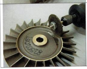
Use a cutting disc in the "Dremel" to perform the grinding. Don't forget to wear your goggles and try to grind away from you as the dust is harmful. If this is tricky to do, then wear a face mask.
