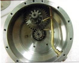
Fit the intermediate gear onto its bearing and fit onto the stub-shaft. Fit the power turbine shaft with its bearing the small pinion gear and M5 nut, and locate into the gearbox
