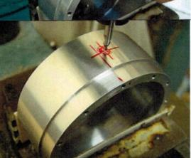
At the 17mm point, mark 3.2mm to the left and at the intersection make a centre punch mark.
