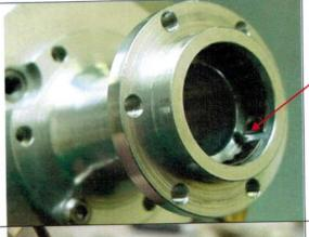
The position of the oil pipe outlet can be seen at left, exiting by the bearing seat.
