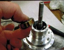
Insert the prop-shaft sub-assembly 162, into the front cover and ensure the bearings are fully seated. Fit the two spring washers 184, back to back as drawn and apply a smear of gasket compound to the front bearing 178. Slide the bearing onto the prop-shaft and into the prop-shaft housing.
