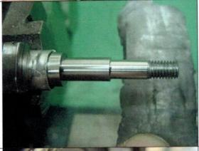
If the fit needs easing a touch more then you need to polish the shaft a little. Use the emery on the back of a fine file and keep checking as you go.
