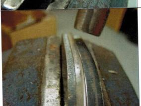
Finally, follow up with a small engineers hammer to flatten down any last small bumps.
