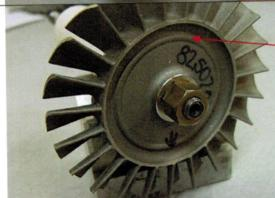
Mark this bottom position and remove the turbine from the shaft. The imbalance must be ground from the ring cast intobeth faces of the turbine.
