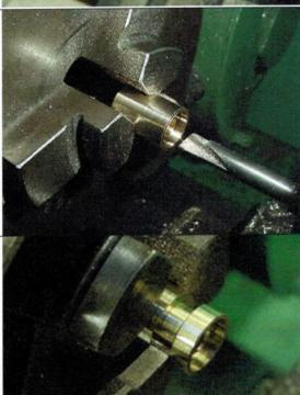
Grip the 10mm brass bar in the chuck, face and centre and drill through 4.5mm.
