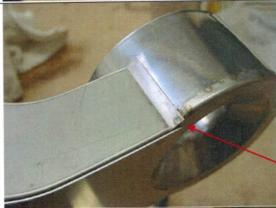
Once in place, apply a couple of tacks at the front end, to hold. Do not tack at the rear edge of the Exhaust-Stack yet as we need to fit the other Stack and align them both into position.
