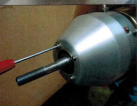
Fit the cowl in place using the eight M2.5 x 5mm securing screws, 189. Use a smear of locking compound on each and tighten evenly. Note, the cowl will push the front bearing back into its working position as you tighten the screws.
