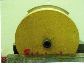
Place the discs together and trap the Exhaust Front between them, aligning the edges carefully. Put an M6 bolt and nut through the centre to hold them together.
