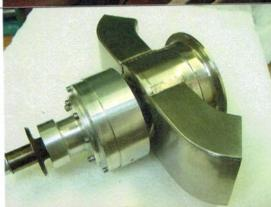
Once welded up, the whole exhaust system can be cleaned up. All welded edges can be smoothed with a fine file or the sanding drum and linisher. Polish up by rubbing over with fine emery to remove the bulk of the scratch and weld marks.
