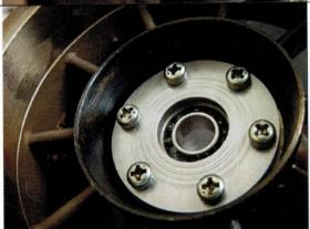
Place the Clamp Ring 143, over the end of the shaft and orientate the holes. The six M3 x 10mm screws 191, can now be fitted complete with their locking washers 199, (note the prototype (left) shows pozi-drive screws but cap heads should be used.
