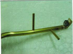
Mark off and drill the two 1.5mm holes for the brass injector pipes. Cut these from a length of 1.6mm (1/16") brass pipe.
