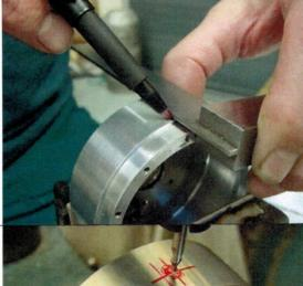
Marking out for the mounting hole.
