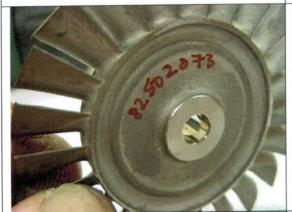
Give the hone a little oil and fit to a cordless power drill and polish the bore slightly to ease it, by spinning the tool and moving it in and out.
