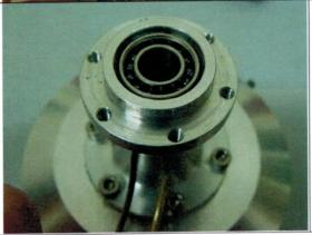
Leaving the shaft in place, apply a smear of low strength liquid gasket compound, available from car accessory stores, to the front face of the shaft tunnel and the underside of the manifold 148. Wait a minute or so for the compound to thicken and ease the shaft tunnel onto the gearbox rear, using the bearing as a peg to ensure perfect centring.
