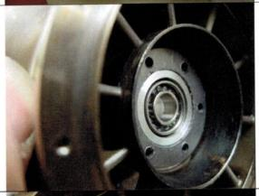
Fit one of the special gaskets 144, into the inner face of the Spider casting, orientating the holes carefully, and slide the whole Spider/Exhaust assembly over the end of the shaft tunnel. Align the holes in the Spider to the shaft tunnel and confirm the correct location.
