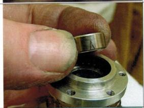
Slide the tolerance ring 185, into place at the turbine end of the shaft tunnel. Carefully insert the ceramic turbine bearing with the arrow pointing out. Gently press this into place by pressing against the outer race – not the centre.
