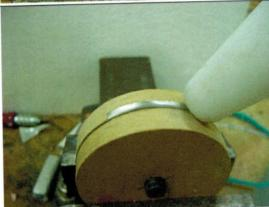
Use a nylon hammer to form the edge over, using small taps and working back and forth along the bend line to keep it even.
