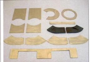
Left shows the laser-cut stainless steel exhaust materials pack, available from Wren Turbines.
