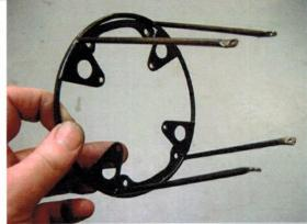
After welding the complete mounting can be cleaned up using files and emery to remove any unsightly lumps and blend the welds neatly. Left, shows the prototype mounting – yours will be simpler as the lugs now have the mounting holes included!
