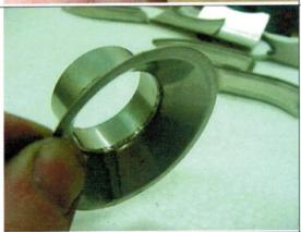
The Exhaust Inner is aligned carefully and spot-welded into place.
