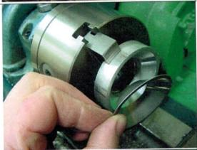
Run your lathe in mid speed (about 350rpm), and use the ballrace to press the edge of the cone flat against the spinning tool, to form a flange.
