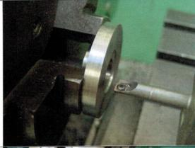
Machine the bulk of the excess material off to get to about 9mm length, then grip on the smaller boss diameter to machine to finish length of 8.5mm.
