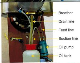
The **breather** pipe needs to finish at the top of the oil tank. The oil **drain line** must be a minimum internal diameter of 3.5mm. The **feed line** connects pump outlet to oil feed connection. The **suction line** connects the tank pickup to the oil pump, via a suitable filter fine mesh filter (not felt). The **oil pump** is a standard fuel-type pump operating on 1-cell switched with a pressure switch, or via an output from the ECU.
