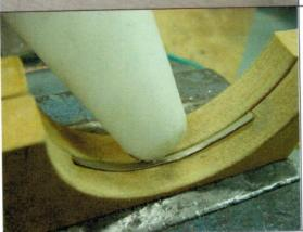
The assembly is clamped into a vice firmly and the flange formed by lightly hammered over with a nylon hammer.
