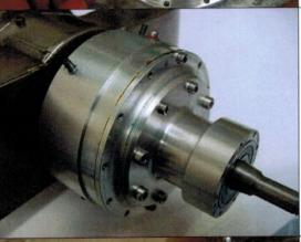
Apply a smear of gasket compound to the front of the gearbox and refit gearbox front assembly, ensuring the intermediate shaft wavy washers are in position.
