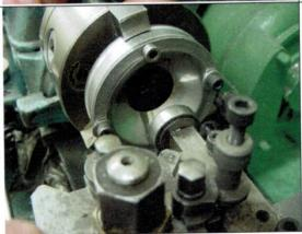
We now need to hold on to the outer diameter of the cone and spin the inner 3mm inwards to form the flange for the exhaust inner. I used an aluminium block with four threaded holes into which I fitted screws and washers to hold the flange. The block was machined with a 10mm recess of 56mm diameter and then a centre hole of 34mm internal diameter was turned.
