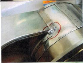
The corner gap sealed with a small TIG weld.
